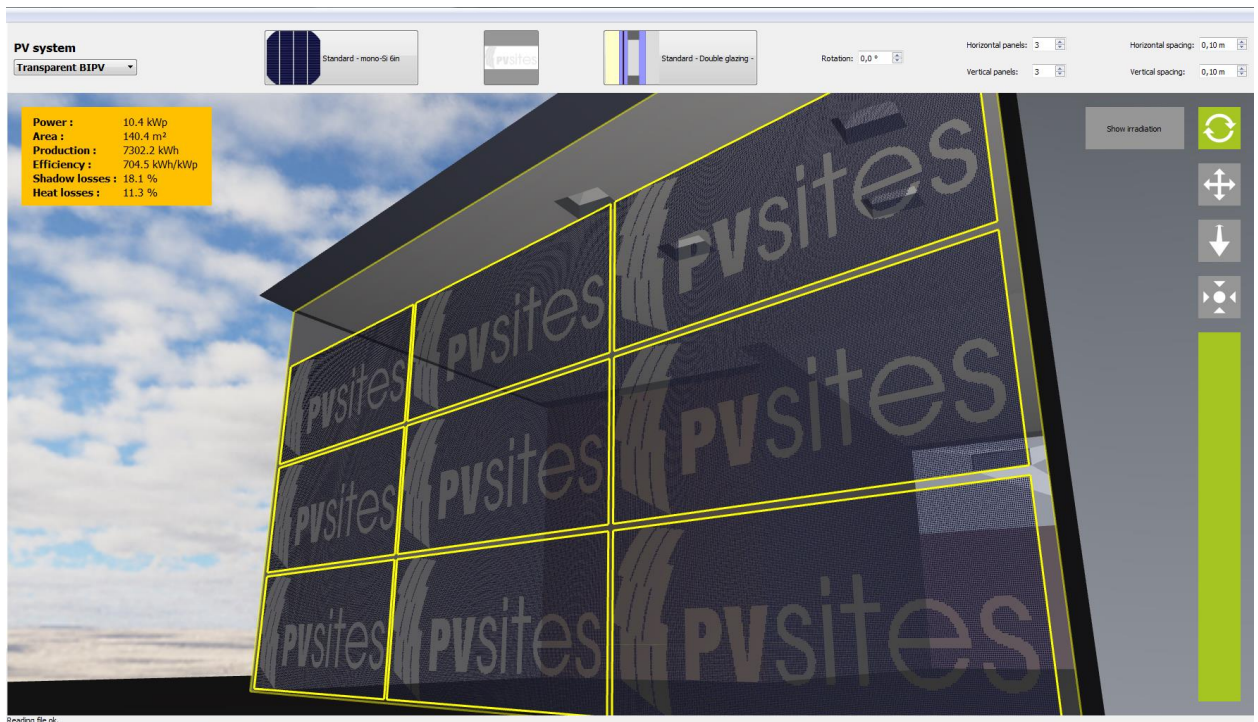
Figure 4.10: PV installation layout, transparent BIPV
