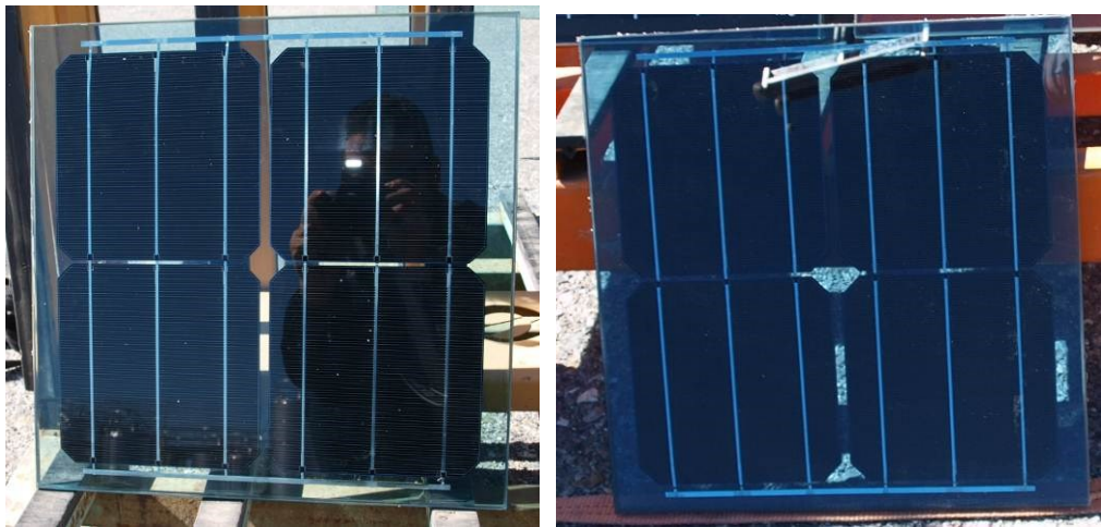
Figure 2.36 Final appearance of samples X12-8 and X12-9 (front views)
