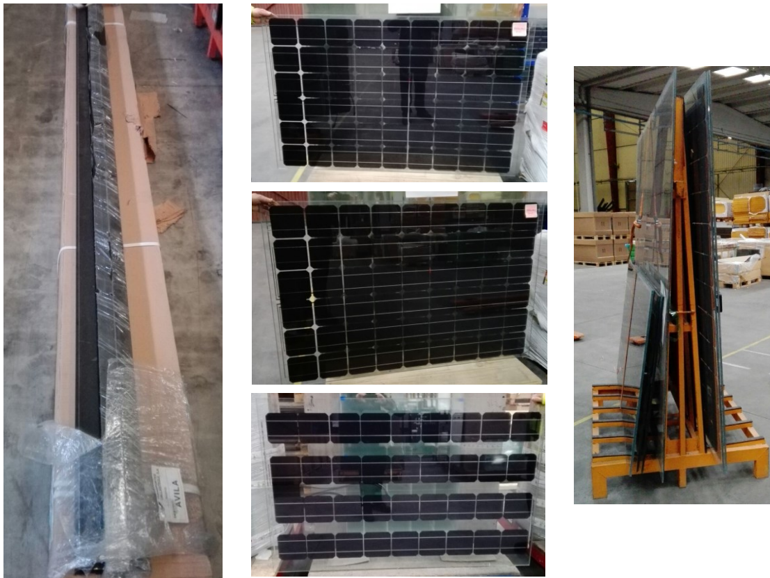
Figure 2.26 Materials for prototype X8-2 (left and center) and support frame containing the PV glass for X8.1 and x8.2
