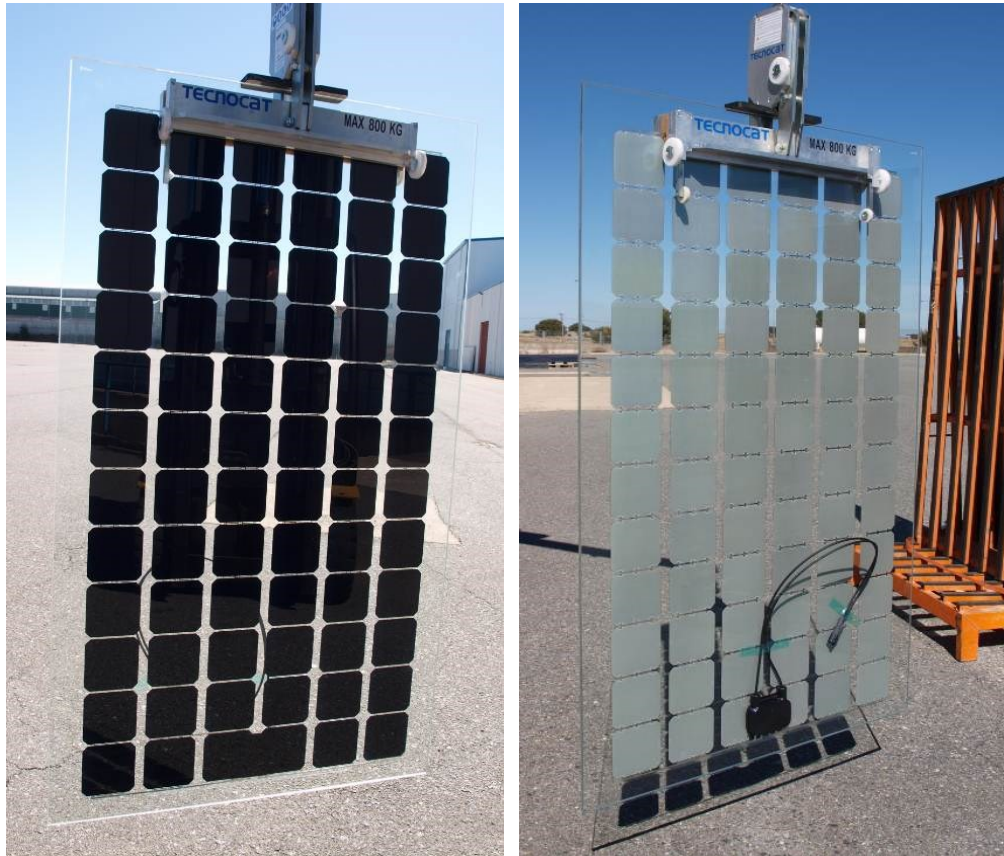
Figure 3.2 Final appearance of the BIPV prototype with back contact cell technology
