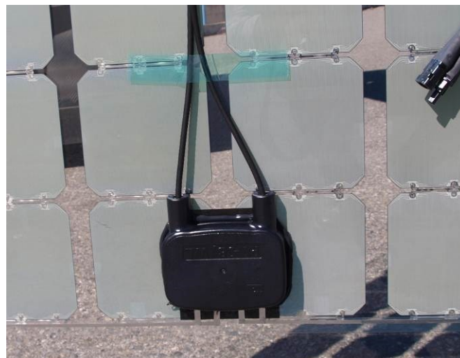
Figure 3.2 Final appearance of the BIPV prototype with back contact cell technology
