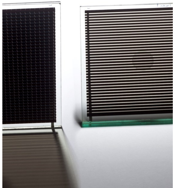
Figure 6.6 Prototypes of PV cells with angular dependency transmission 2011 (Signet Sola)
