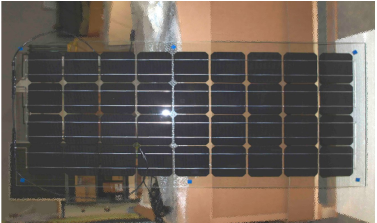
Figure 9.17 c-Si large area glass module
