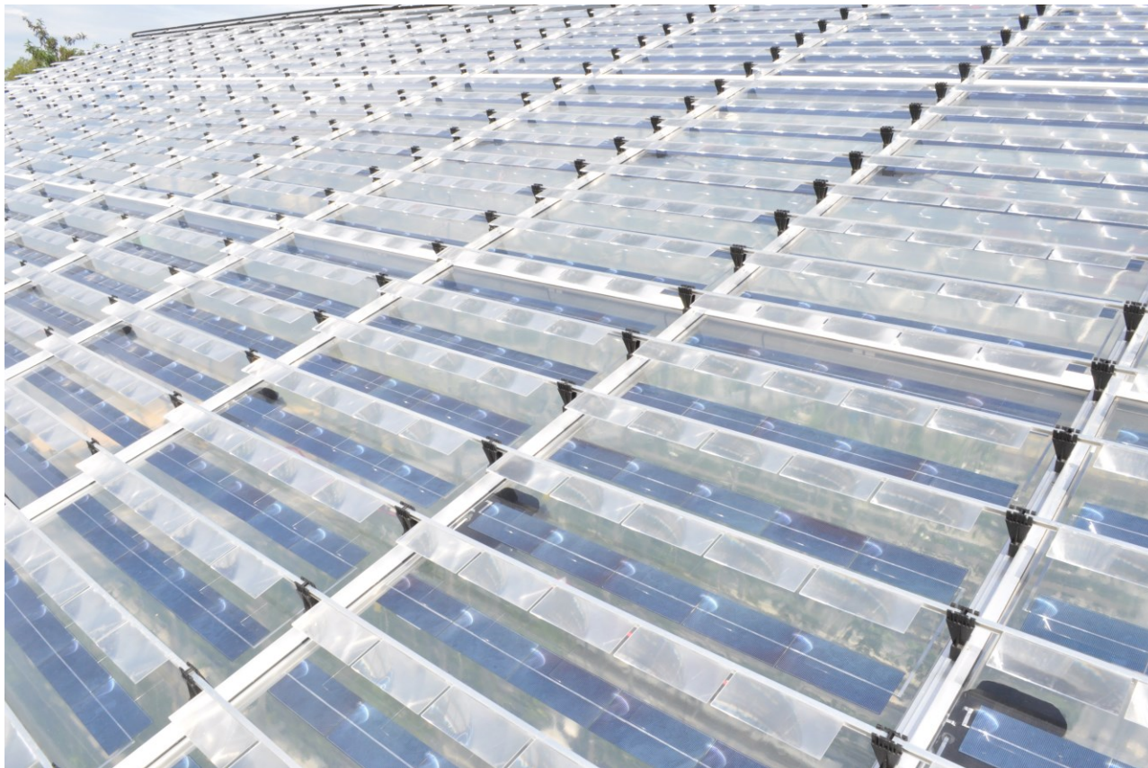
Figure 9.20 Test site with c-Si semi-transparent, low concentration roof in a greenhouse
