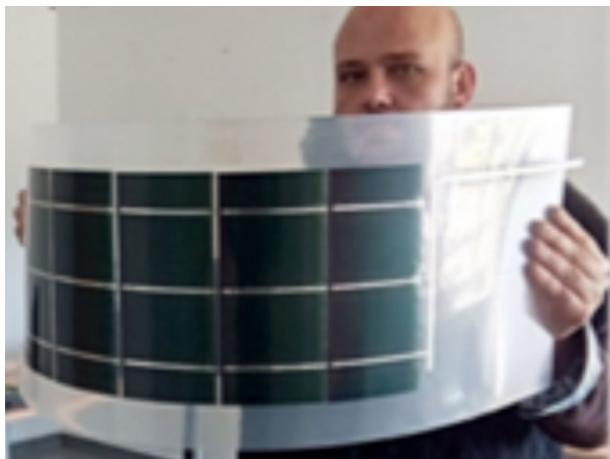
Figure 9.15 and Figure 9.16 Example of internal sheet of curved CIGS element
