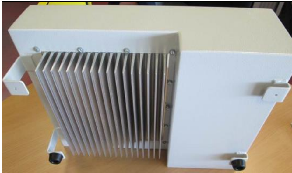
Figure 9.4: Back view of the inverter with heatsink and wall mounting system
