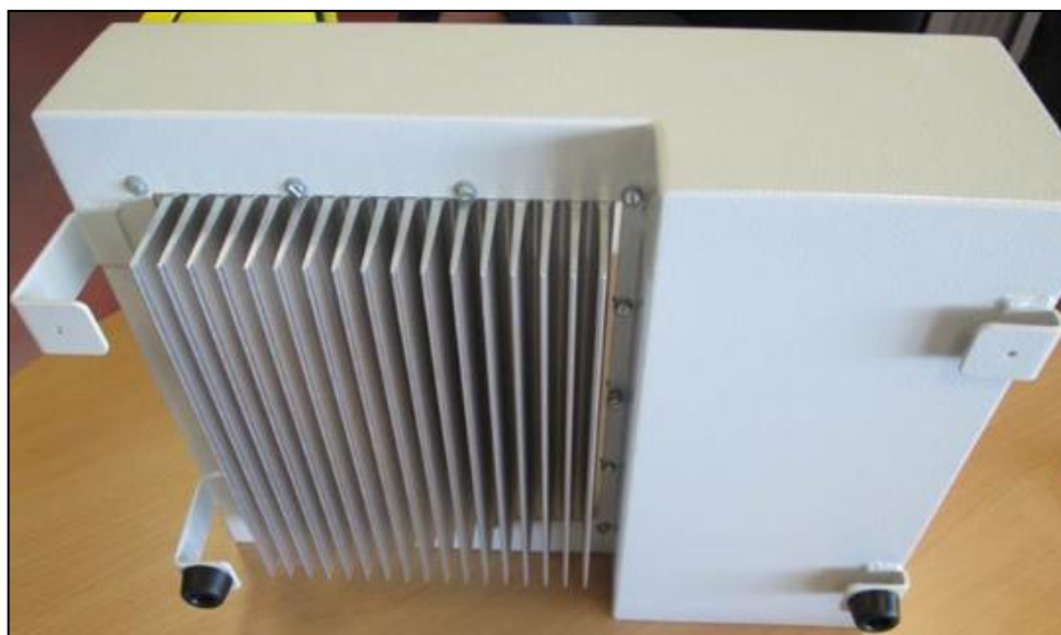
Figure 8.4: Back view of the inverter with heatsink and wall mounting system
