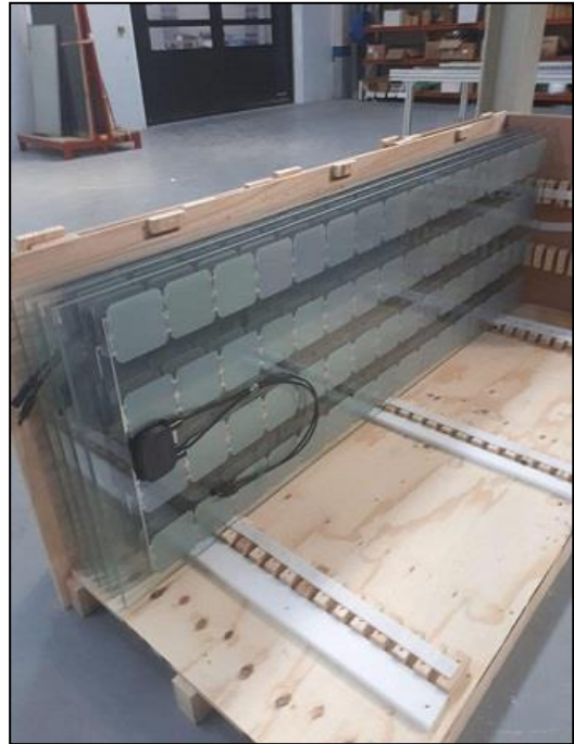
Figure 7.7: X6 c-Si back contact modules stored in crates and ready to be shipped
