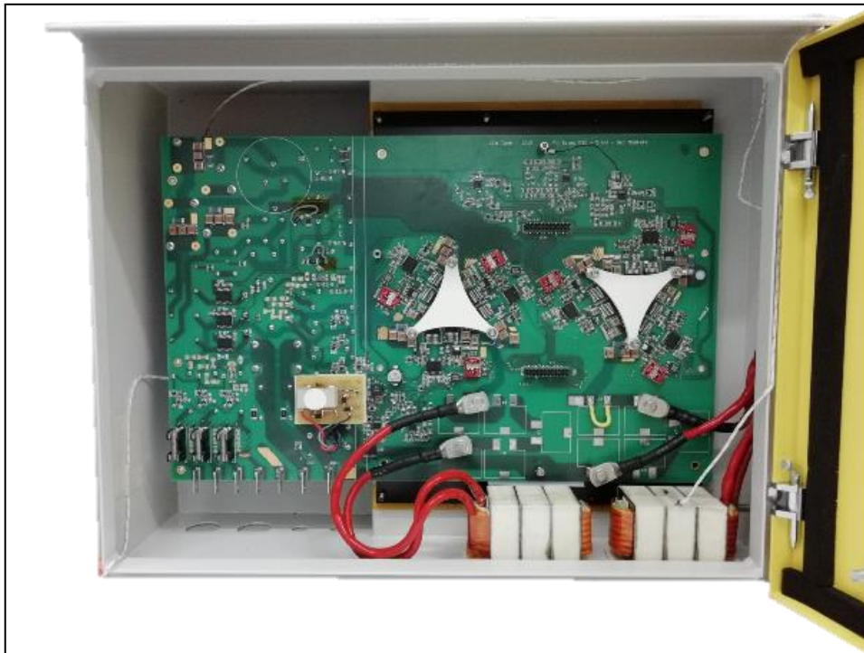
Figure 8.5: Printed circuit-board placed into the housing
