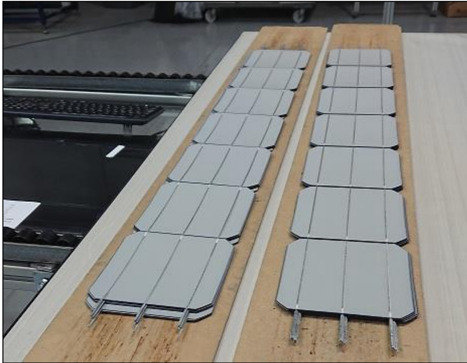
Figure 6.3: Detail of strings of cells
