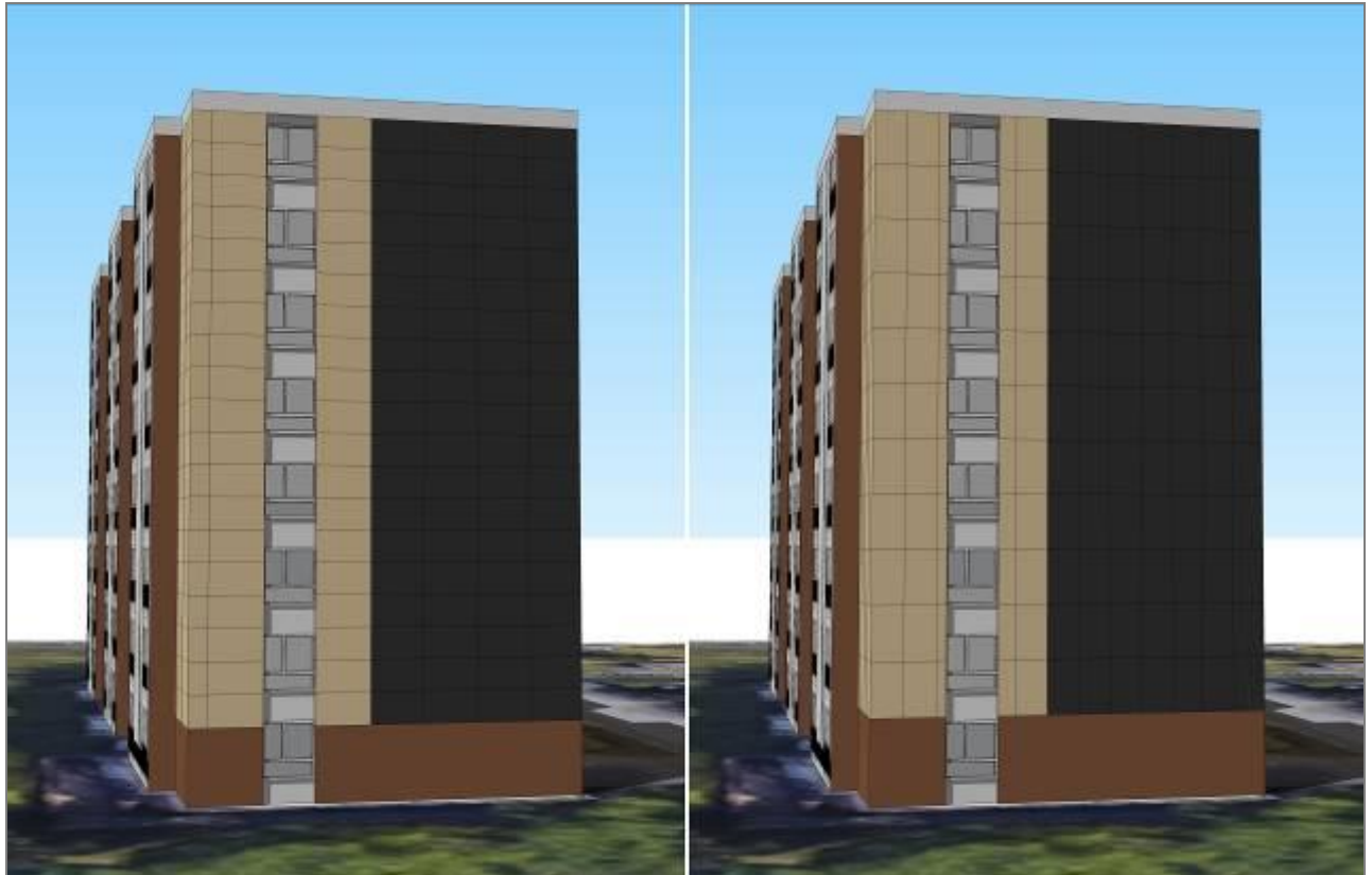
Figure 3.42: Horizontal and vertical options (1st proposals) related to the layout of the modules
