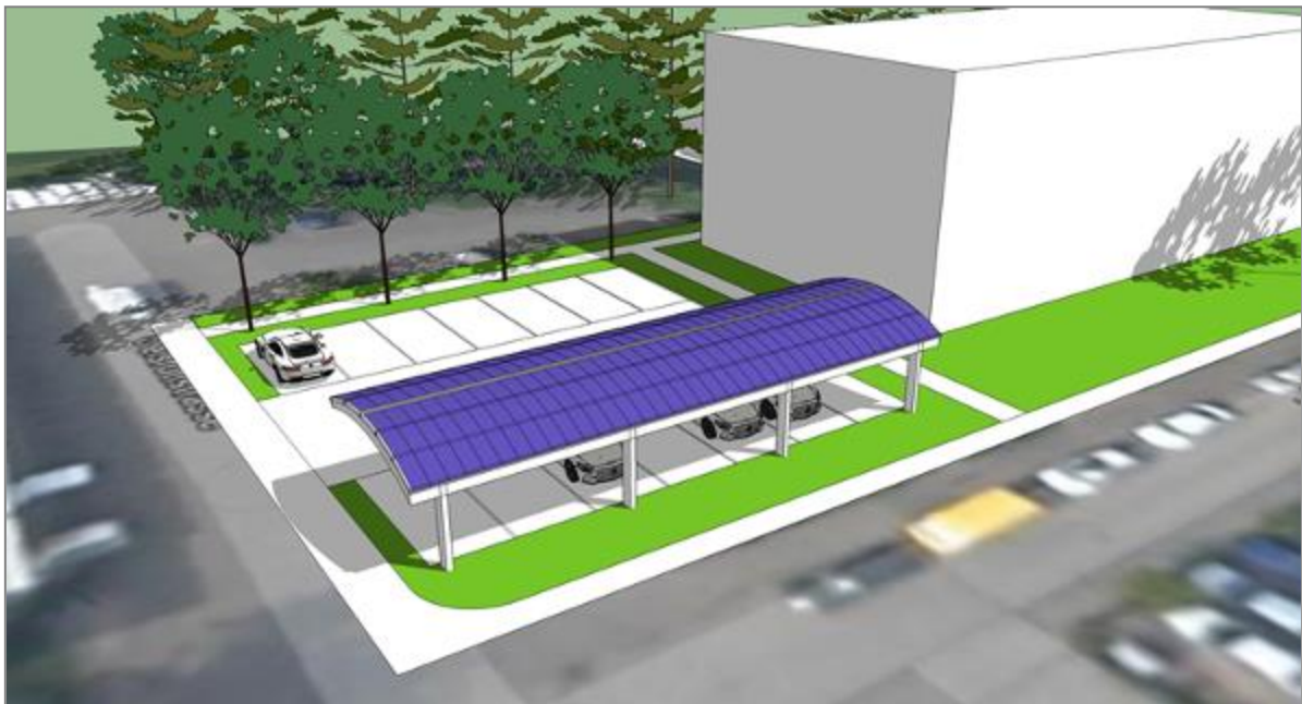
Figure 3.27: PV carport at EKZ facilities
