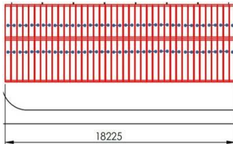
Figure 3.22: String concept for EKZ's carport
