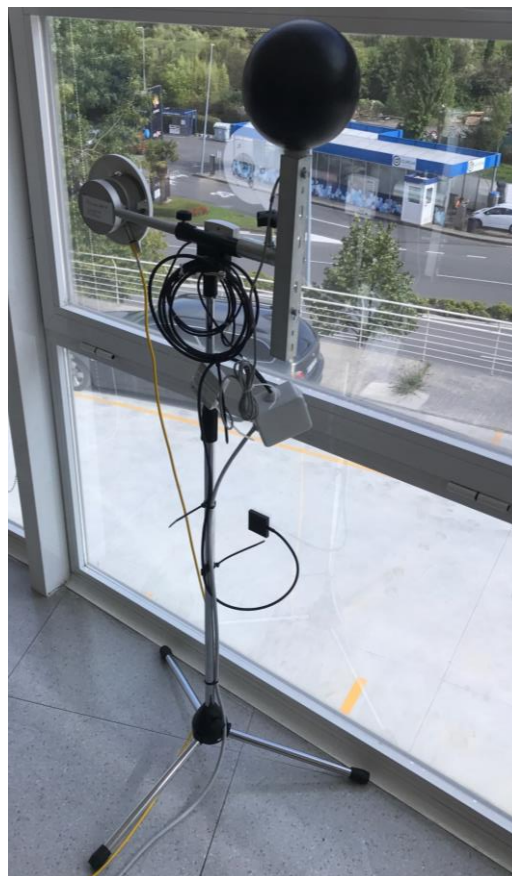
Figure 3.25 Operative temperature sensor, air temperature + relative humidity sensor, and luminance sensor installed in the buffer area located behind the window where the BIPV system will be installed
