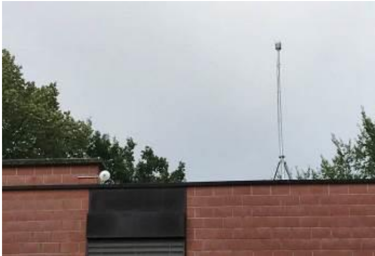
Figure 3.7 Weather station and pyranometer installed on the roof of Pavilion 2
