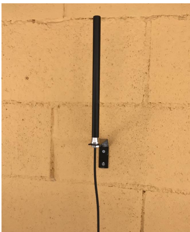
Figure 3.15 Remote antenna for communication with wireless T/RH sensors
