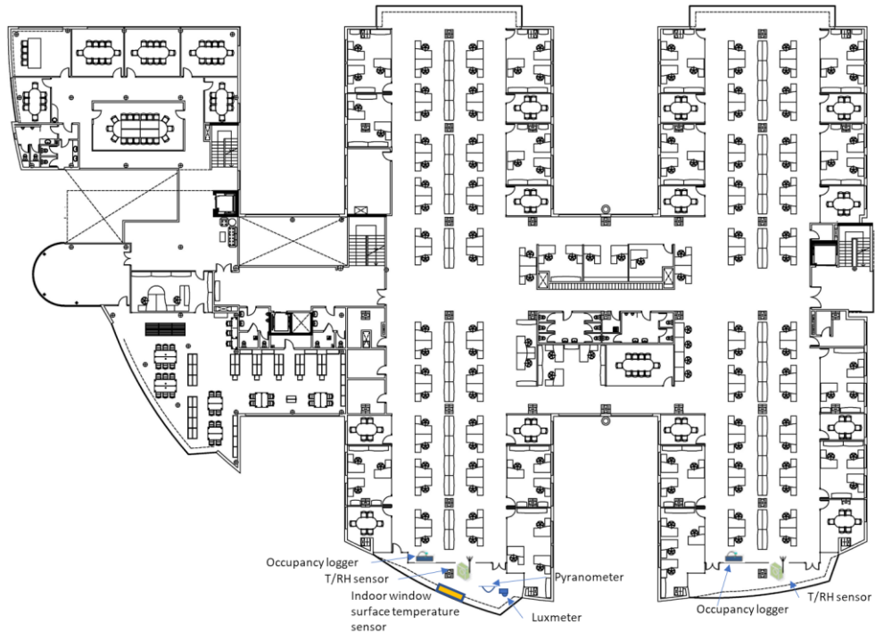
Figure 3.26 Location of the sensors on the first floor of the building
