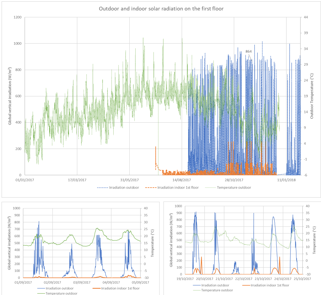
Figure 3.57 Indoor and outdoor solar radiation measured in the room located behind the glass façade on the first floor
