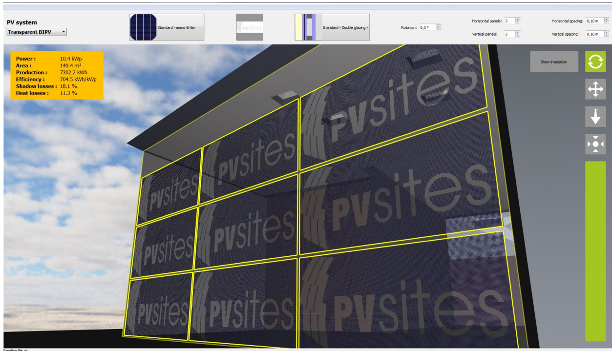
Figure 17: PV installation layout, transparent BIPV
