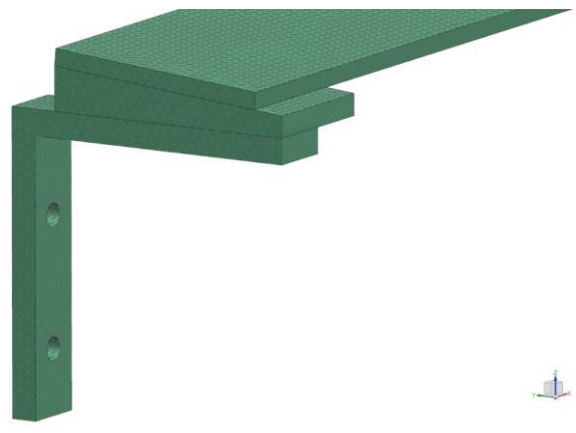
Figure 4.34: Detail of the finite element mesh of the lamella
