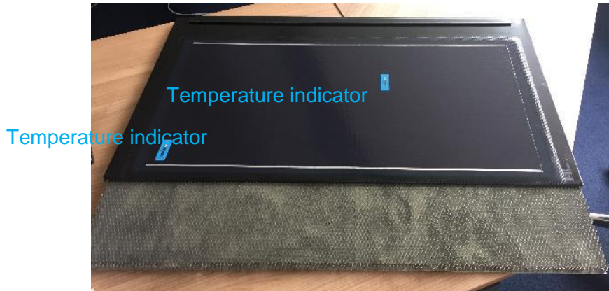
Figure 2.1: Roof tile lamination prototype. This prototype was used to verify the lamination process compatibility for temperature and mechanical stability.
