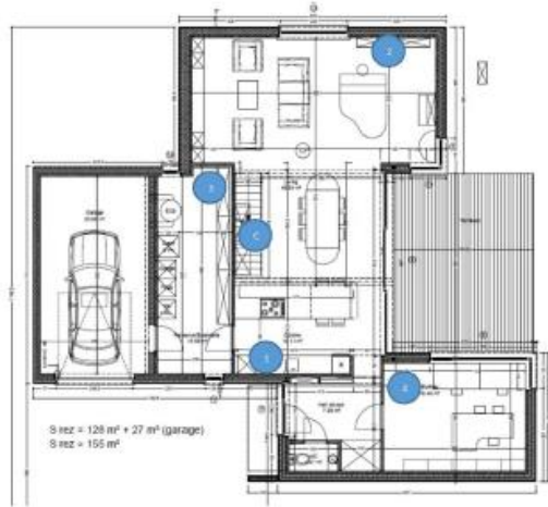
Fig. 7.4: First floor, Temperature and Humidity sensors position
