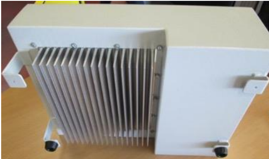
Back side of the inverter
