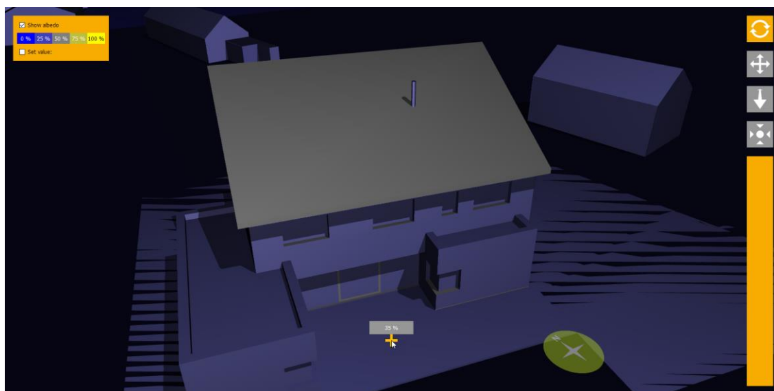
Figure 4.9 Albedo effects (reflected irradiance) are generated selecting groups and types of surfaces
