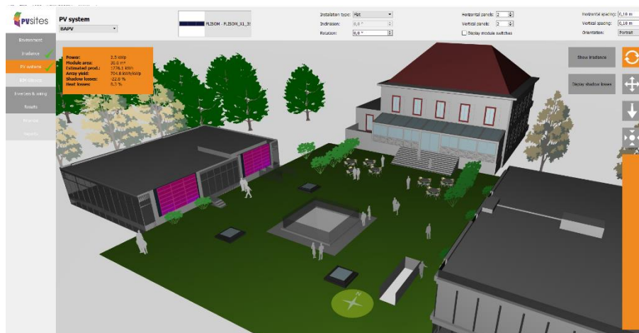
Figure 4.26 Production on Pavilion 1 (West facade). KPIs: Power=2.5kWp (30sqm); Array yield=705kWh/kWp; Total production=1,776kWh/y; albedo effects are huge and enable production (22.8%)
