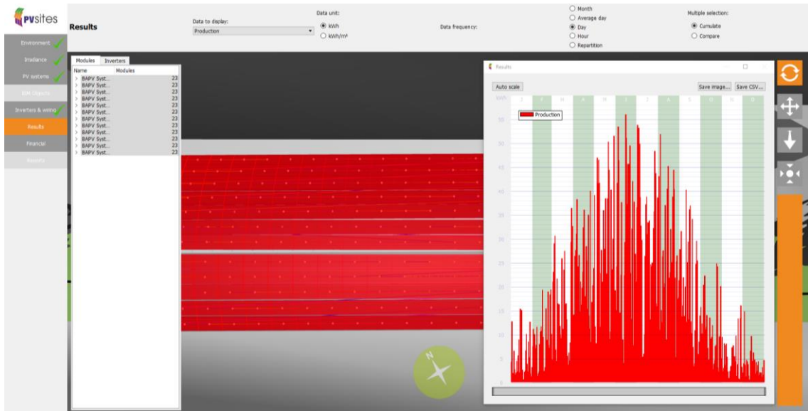
Figure 4.43 EMPA Carport - Up: average daily production; Down: Hourly production; csv exportation to downstream processing (PVSITES planning tool)
