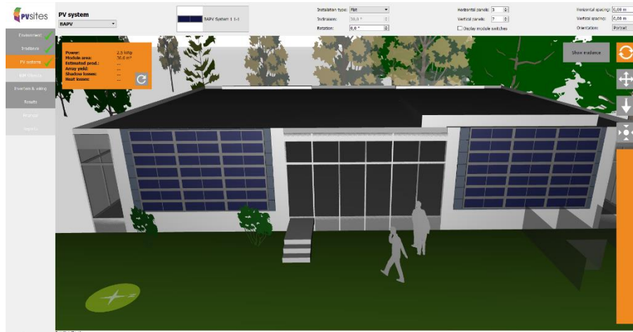
Figure 4.25 PV layouts on Pavilion #1: 2 distinctive layouts of 1x2 FLISOM X2 60Wp modules – BAPV mounting
