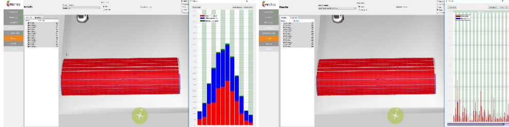
Figure 4.39 Left: Yearly Irradiance: direct / diffuse / indirect. Right: Hourly production; csv exportation to downstream processing (PVSITES planning tool)
