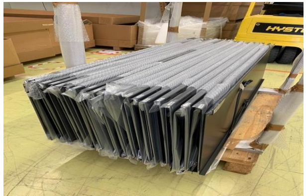
Panels being packed after PV lamination for shipment to Ernst Schweizer AG
