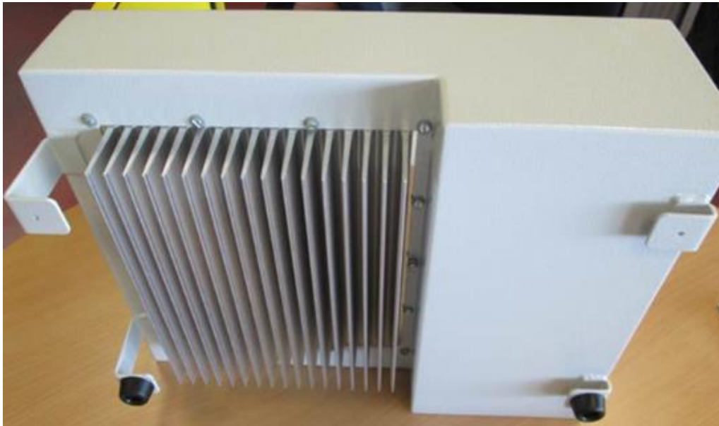
Back side of the inverter
