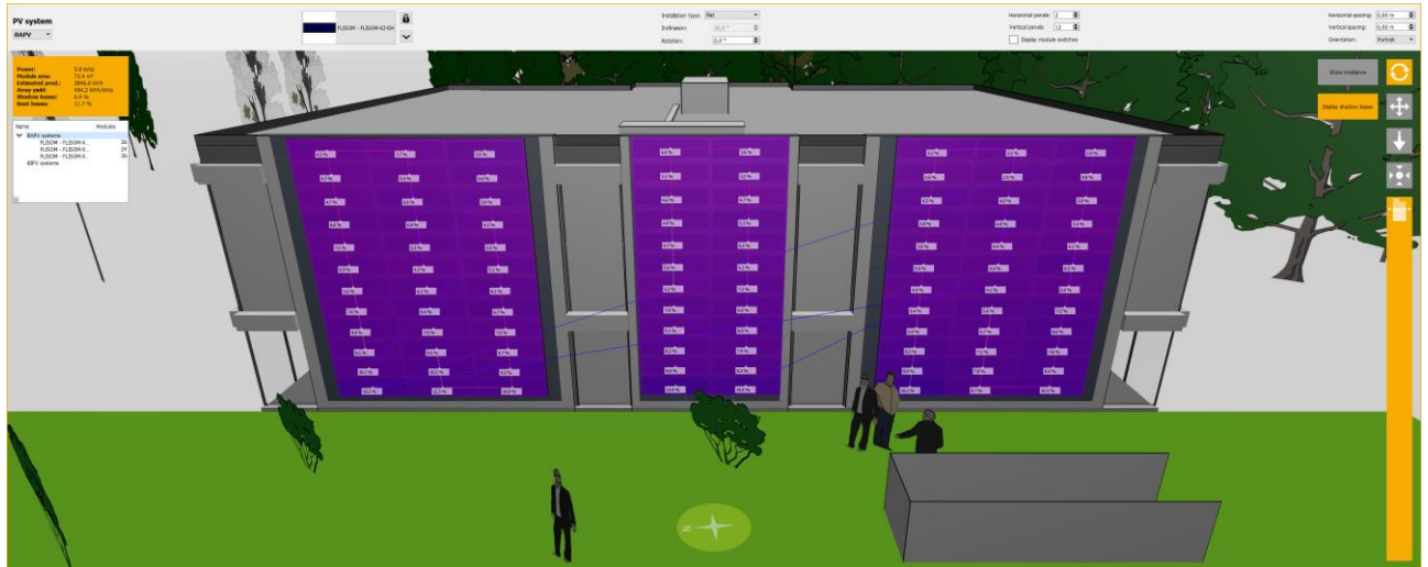
EHG Pavilion 2 - PV Production + shadow losses + Yield – Hourly step / Module level
