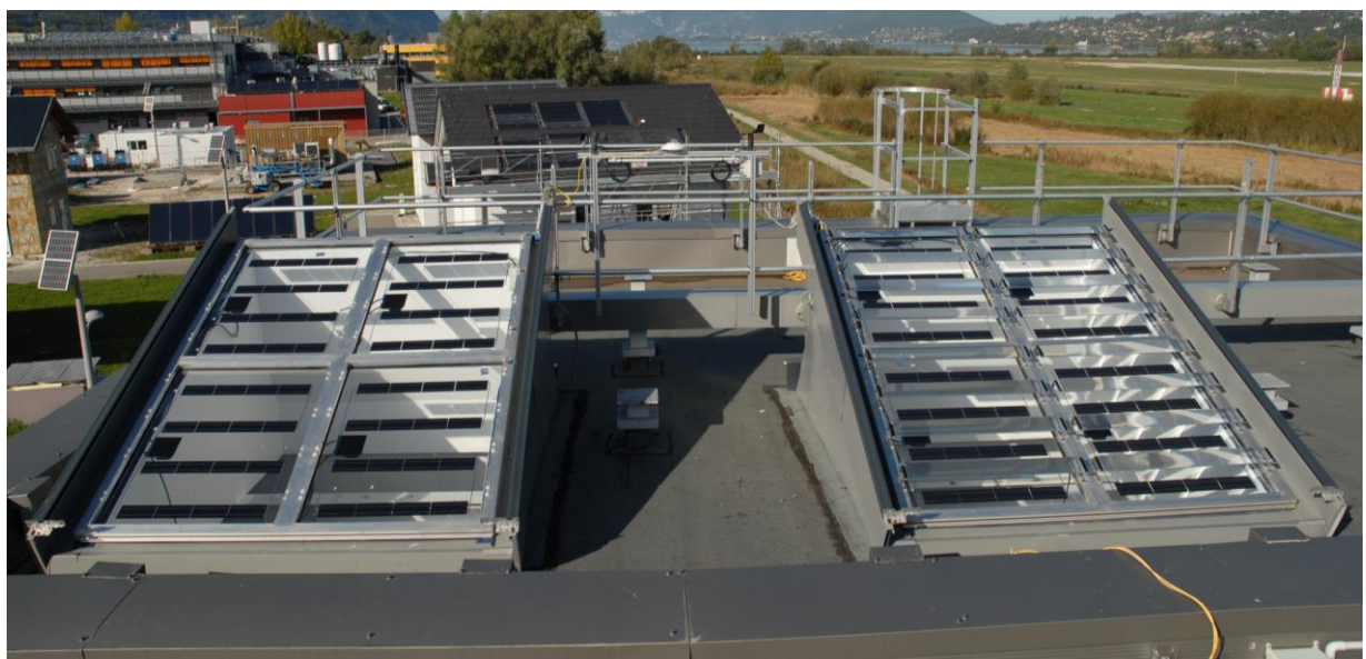
Two PV skylights installed in FACT experimental building at CEA-INES, Chambéry, France. Left : Reference PV skylight without lenses (REF) Right : New PV skylight with lenses (LCSK)
